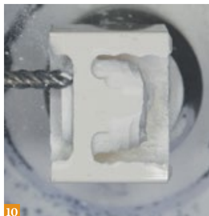
FIG. 10: The gross reduction of the TZI C block is removed by the Shaper 25 bur. Note the dry milling of the block.
