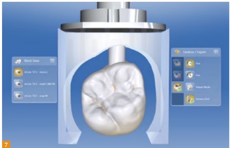
FIG. 7: The mill preview of the restoration. You can see the option to fast mill the zirconia. My experience is that it results in wonderful milled margins. You also can see that the furnace is automatically selected so the software knows to transfer the sintering parameters automatically after the milling process is complete.
