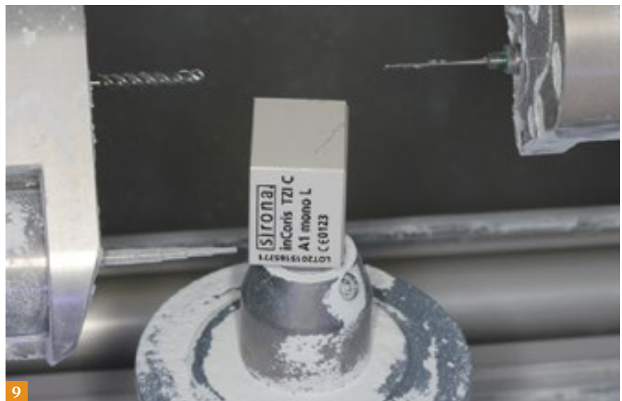
FIG. 8: The time it takes to fast-mill a zirconia restoration is just over 10 minutes — milling approximately as fast as other CEREC ceramic materials
